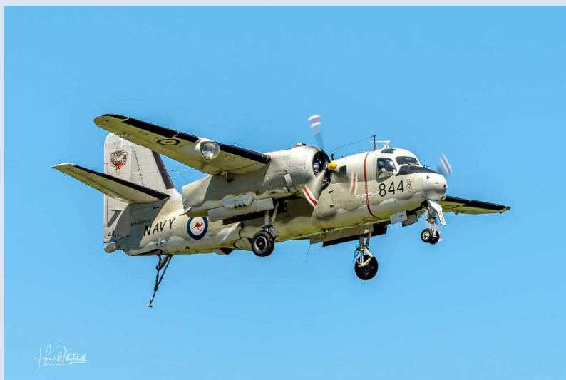
Grumman Tracker – configured for arrested Aircraft Carrier landing.
