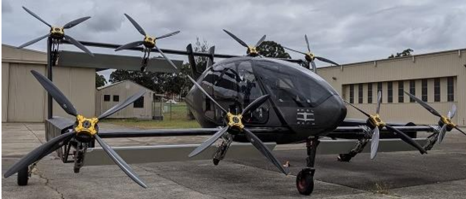
AMSL Aero – Vertiia, electric/H 2 Tilt rotor
