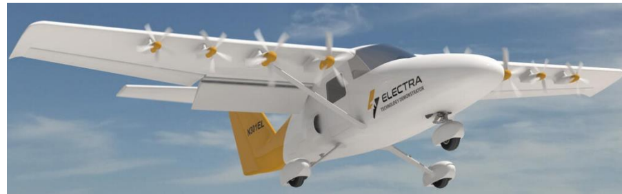
Electra Aero – blown lift, eSTOL
